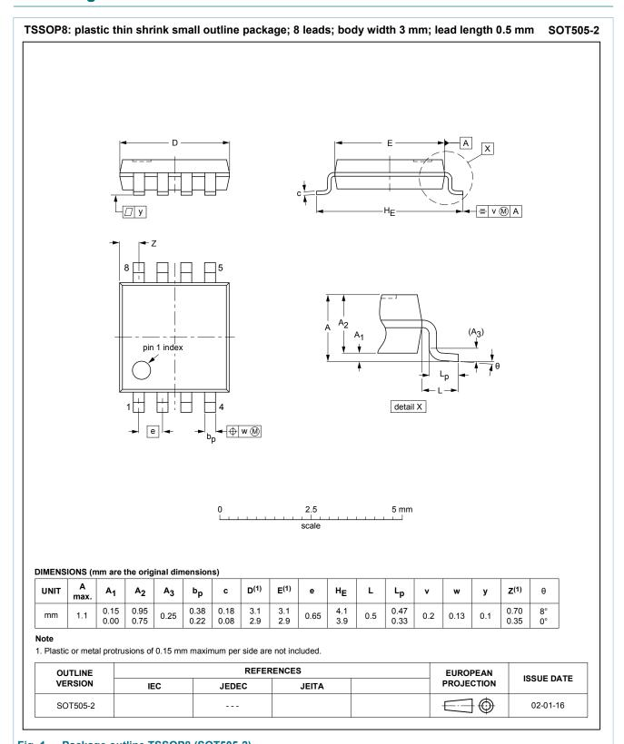
plastic, thin shrink small outline package; 8 leads; 0.65 mm pitch; 3 mm x 3 mm x 1.1 mm body
